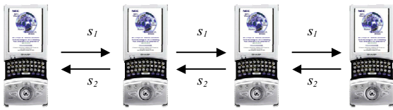
Fig.5. SCP demonstrator set-up with four Sharp Zaurus PDAs to measure round trip times, jitter and throughput.
