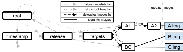
Figure 3: The four basic (root, timestamp, release, and targets) roles used in TUF.
